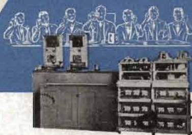
1914. World's first vacuum tube repeater amplifier; designed by Bell Telephone scientists and made by Western Electric for transcontinental telephony, was the start of modern electronic communications.
